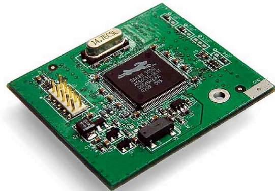
Figure 1-12 - The Jackrabbit RCM3100 core module, which is the microcontroller used for the Cool Robot. [Z-World 2005]
