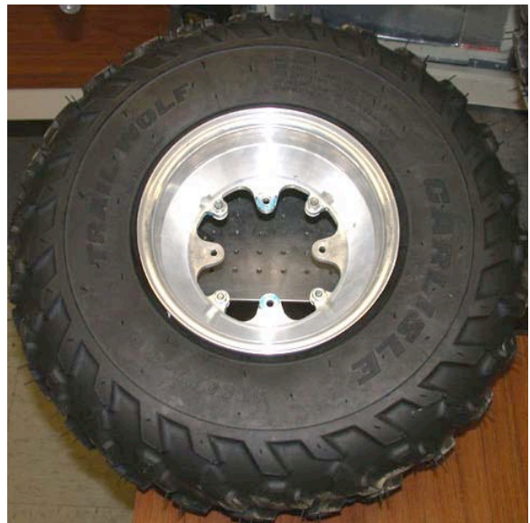
Figure 1-11 - The custom machined aluminum wheel with a 20x8 ATV tire mounted to it.
