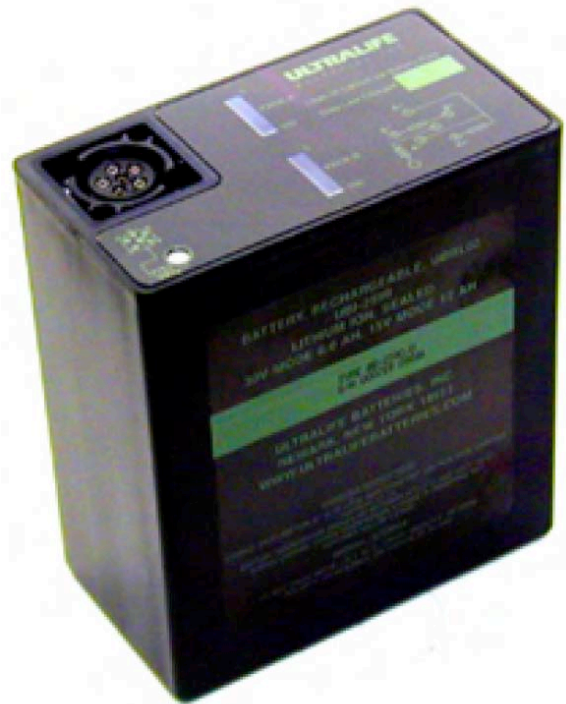
Figure 3-30 – The Ultralife 2590 Lithium-Ion battery used in the Cool Robot.
