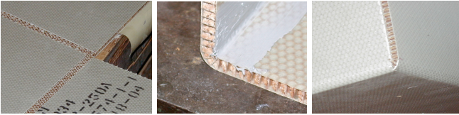
Fig.5 Chassis fabrication using fiberglass-Nomex honeycomb composite
