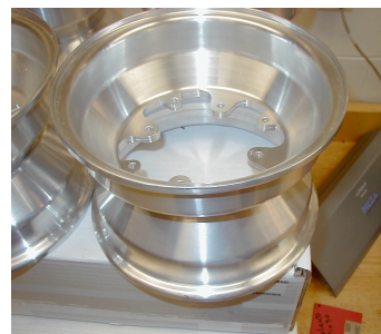
Fig. 4 Custom rim designed for 20x6-8 or 16x6-8 ATV tires
