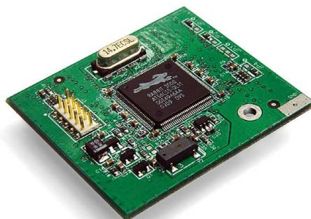
**Figure 6.2:** *Picture of Z-Worlds RCM3100 core module*
