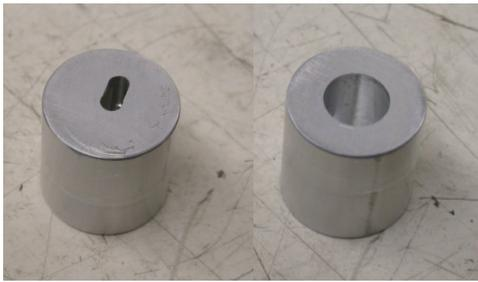
**Figure 2.5:** *The aluminum shaft collars*
